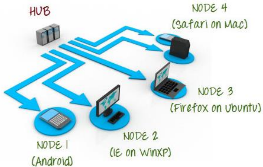
Figure 1. Selenium Grid uses a hub-node concept where you only run the test on a single machine called a hub , but the execution will be done by different machines called nodes
